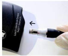
Figure 9: handpiece and device cable
